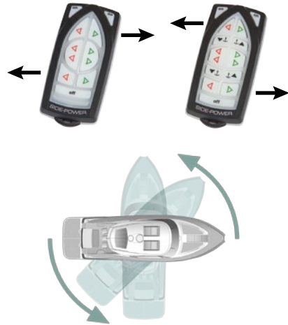
Activating both bow and stern thruster to rotate the boat on axis
