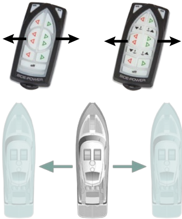
Activating both bow and stern thruster to push the boat sideways
